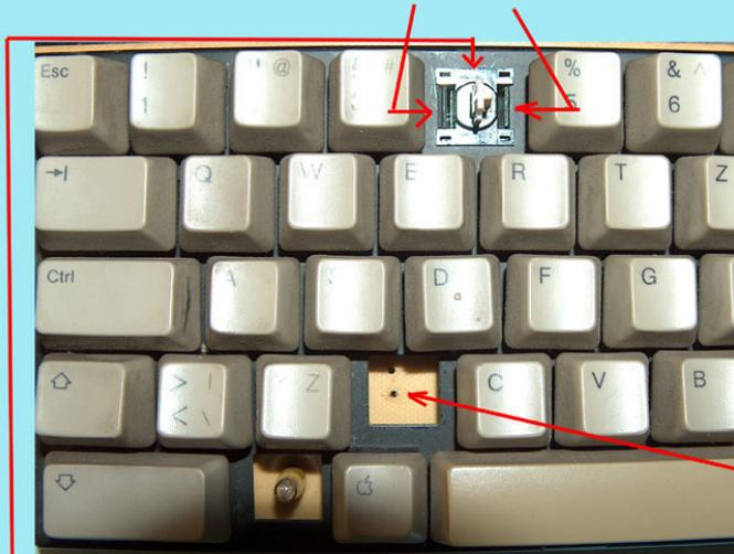
you then must lift gently the switch by slipping with a blade or other very flat tool below the plastic-collar of the switch and lifting up till the keyswitch flips upward. Then the key can be pulled gently off from the PCB.
