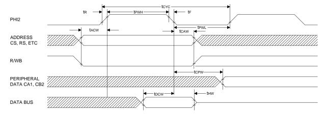
Figure 4-2 Write Timing
