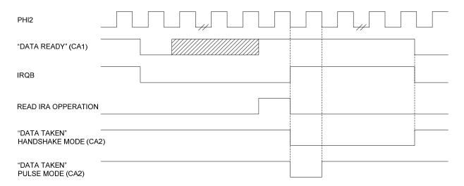
Figure 2-1 Read Handshake Operation (PA Only)
