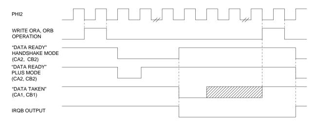
Figure 2-2 Write Handshake (PA and PB)
