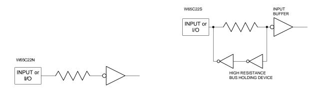
Figure 5-2 High Resistance Bus Holding Device
