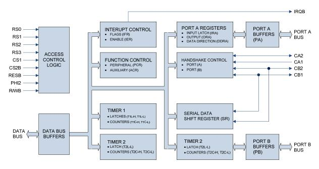
Figure 1-1 W65C22S Internal Architecture Block Diagram
