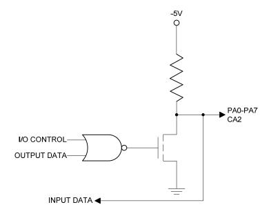
Figure 3-10 Rockwell – R6522 NMOS Port A Buffer Circuit
