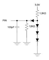
Figure 4-12 Test Load (All Dynamic Parameters)
