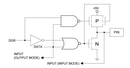
Figure 3-7 W65C22N GTE - G65SC22 CMOS Port B Buffer Circuit
