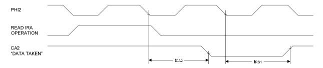
Figure 4-3 Read Handshake, Pulse Mode (CA2)
