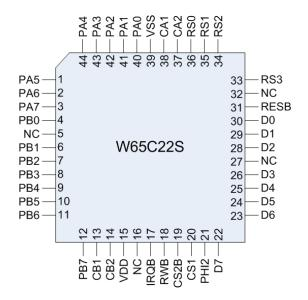
Figure 3-3 W65C22S 44 Pin QFP Pinout
