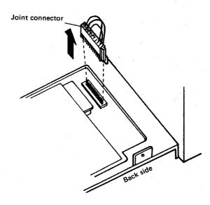
(4) Plug the connector of the MZ-1T04 data recorder onto the pins which were left open when the joint connector was removed in step (3). When doing this, be sure the connector is oriented properly.
