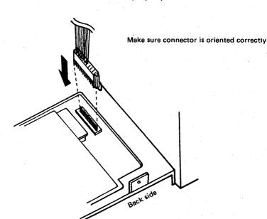
(5) After plugging in the data recorder connector, position the data recorder on the MZ-811 and fasten it in place with the two screws. When doing this, ensure that the flat connector cable does not become pinched between the data recorder and the cabinet of the MZ-811. (Otherwise, it will not be possible to fasten the screws properly.)
