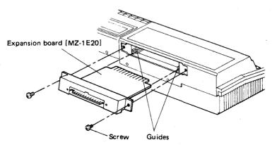
3. Connect the expansion unit connecter to the expansion board and screw both ends of the connecter.
