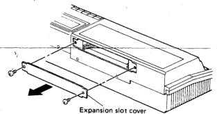
2. Insert the expansion board along the guides on both sides and firmly insert it into the connecter mounted inside the slot. Affix it with the two screws to the rear panel of the MZ-800.
