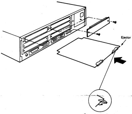
For removal, pull out in direction of arrow so that the ejectors can stay up.
