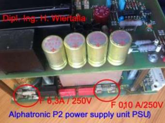
The fine protections (FUSE) examine. In the PSU are <u>three</u> fine fuse (in my machine).
