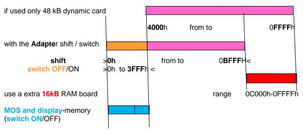
**After RESET** the MOS and the display memory is aktiv = ON. Used with the Adapter the first 16 kB from the dynamic memory is deaktiv = OFF. (top)
