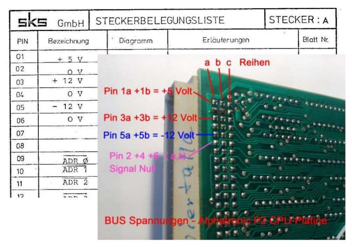
If three DC voltages are to be seen OK, however, no start sequence on the screen, the boards are other to examine like here.
