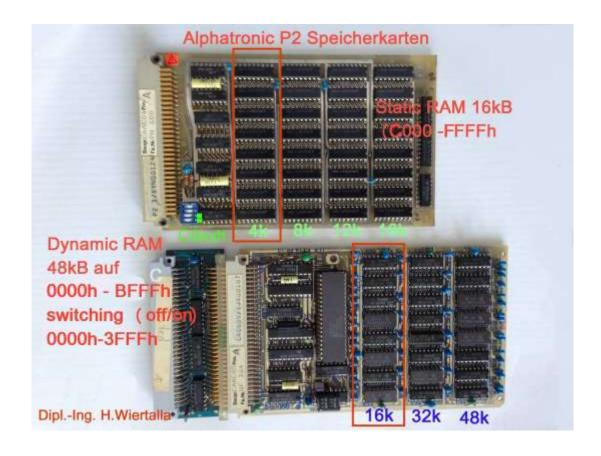
If you used **only the 48kB** dynamic memory card, then is the ADDRESS 4000h to FFFFh. Only for 4300H TPA cp/m, or other software for running 4000h between FFFFh !!! (top)
